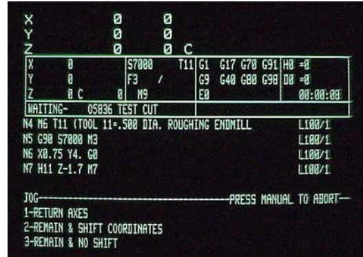
Figure 4-1 The control in waiting mode.
