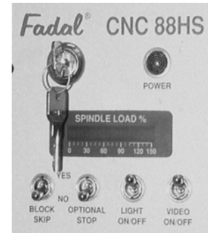
Figure 2-3 KEY LOCK used to protect unauthorized editing of programs.
