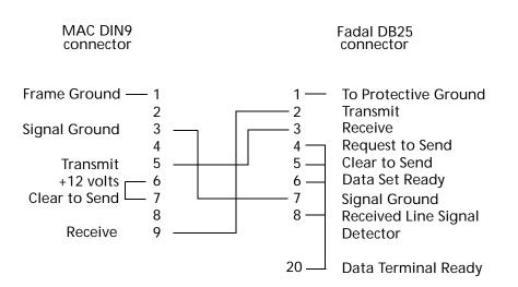
*Note:* Connect pin one to the shield only at the machine end.
