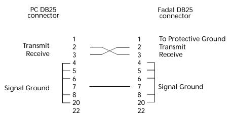
*Note:* Connect pin one to the shield **only** at the machine end.
