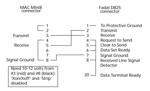
*Note:* Connect pin one to the shield **only** at the machine end.
