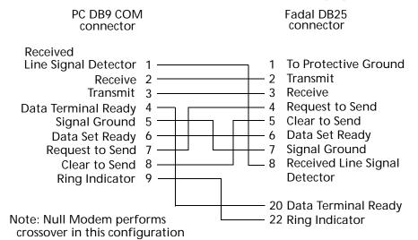
*Note:* Connect pin one to the shield **only** at the machine end.
