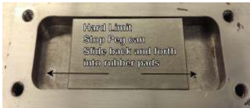
Illustration 1: The hard stop installed
