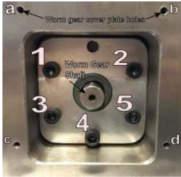
Figure 1: Holes a, b, c, & d cover the worm gear shaft. Screws 1, 2, 3, 4 & 5 hold worm gear shaft in place.
