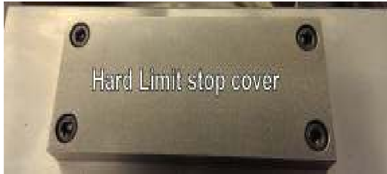
Illustration 3: Hard stop cover. Remove only if table can't be rotated off the hard stop.
