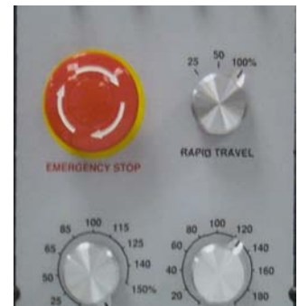
Figure 5-1 Emergency stop button.
